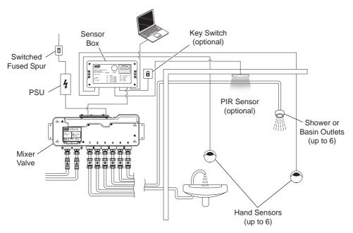
Installation Schematic Diagram
