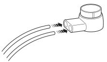
2. Using a pair of pliers, compress the connector to complete the connection.
